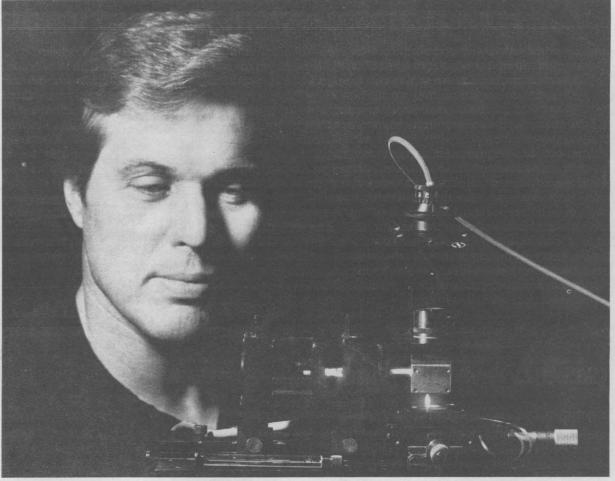
BLOOD LASER — Paul Gourley examines a semiconductor diode laser's horizontal and then bent vertical beam used to excite his VCSEL biocavity laser. The VCSEL releases an invisible infrared beam carrying information about blood cells to a detector, above. (Photo by Randy Montoya)
